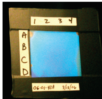
Figure 1. 3 cm \times 3 cm TGCCA fabricated between glass plates by using a 100 \mu m thick polyester spacer to separate the TGCCA from the adhesive used to seal the edges of the glass plates. The cell was divided into 16 9 mm square regions (A1–D4) that were analyzed via UV–vis transmission spectroscopy by using a 5 mm diameter aperture.
